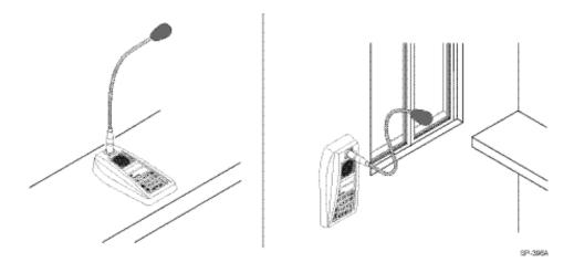
Figure 4. Suggested Selector Station Placement
